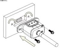
Type 2 Step1: Assemble logger to the inverter communication interface as shown in the diagram.
